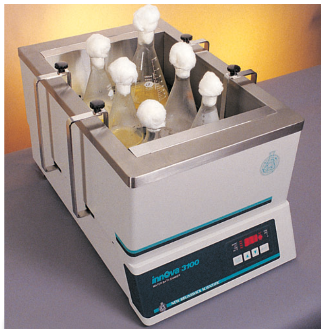
Innova 3100 high-temperature water bath shaker.
